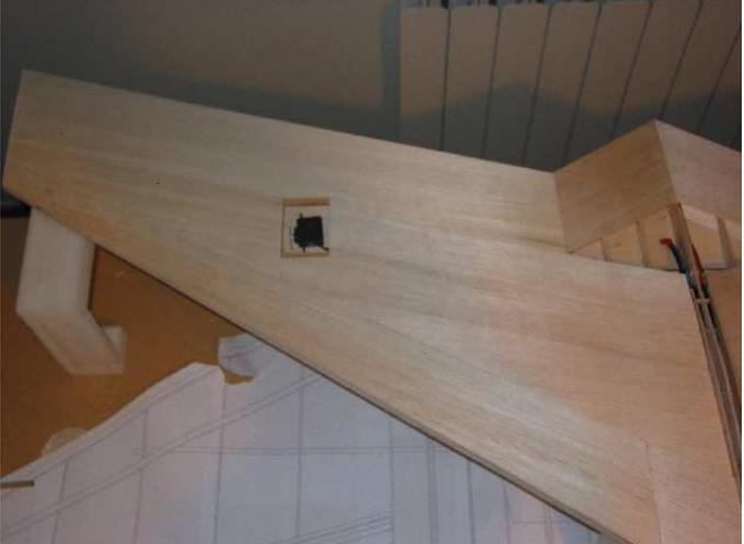
A close-up photograph of the left wing structure. The wing is made of light-colored wood. A small, dark rectangular opening is visible in the upper part of the wing, which is the area where the servo tray will be installed. The structure is supported by a white foam block. |
